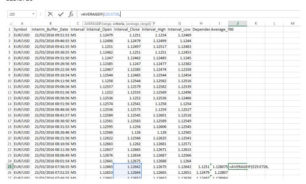
The next parameter of the AVERAGEIF is the string representing the filter. This string will be a concatenation which will include a condition and the cell value of the Interval\_Close, as cell E25, constructed as follows:
