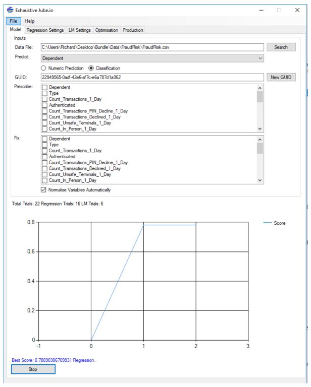
The model will keep running ad infinitum, or until the maximum number of trials is exceeded as specified in the Settings tabs. In this example, the best score achieved is 78, which would indicate that the average between Correlation and Percentage Correct is 78.
