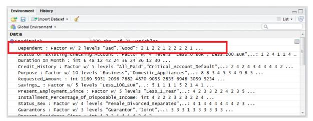
It follows that predictions that are closer to 2, than 1 would be considered to be Good, whereas vice versa, 1. To appraise the model performance, a confusion matrix should be created. Create a vector using the ifelse() function to classify between Good and Bad:
