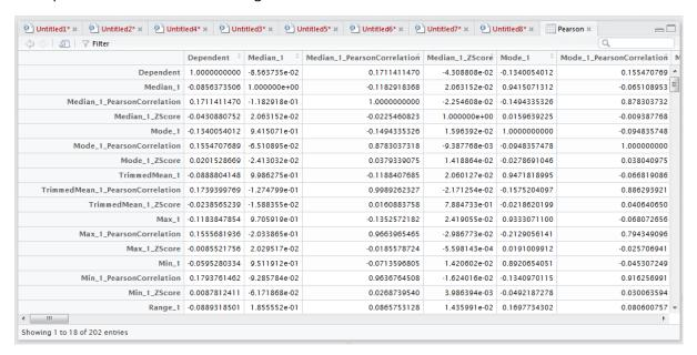
The task is to use matrix logic to identify correlations which exceed 0.7 or is below -0.7 (as both extremes of +1 and -1 are equally troubling in this example). The statement will use the or operator (i.e. |) and create a new correlation matrix:
