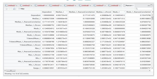
As the Pearson correlation is a matrix object, it can be interacted with via subscripting. While the correlation matrix is extremely useful for identifying collinearity, at this stage the main point of interest is the relationships to the dependent variable only.
