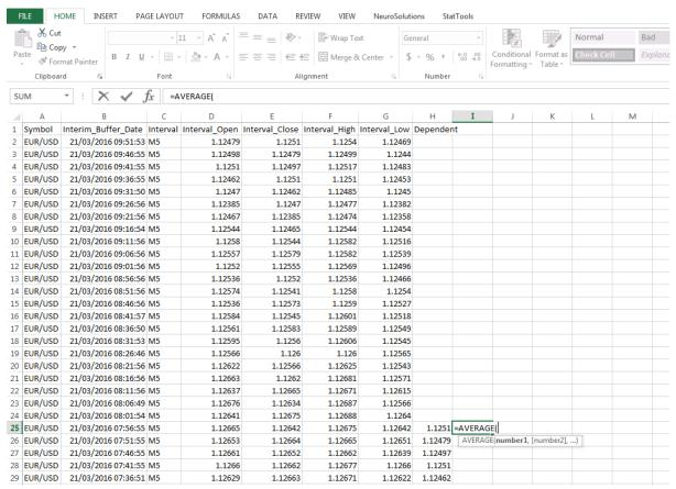
In this example, the scope is the last 700 intervals backwards. Therefore, taking the Interval\_Close column, which is Colum E and excluding the first 24 examples which are not complete, the scope can be described as being all cells in column F between 25 to 726, or rather:
