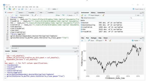
This procedure should exhibit that qplot has default of a scatter chart, however it can be easily changed to other types by varying the geom parameter.
