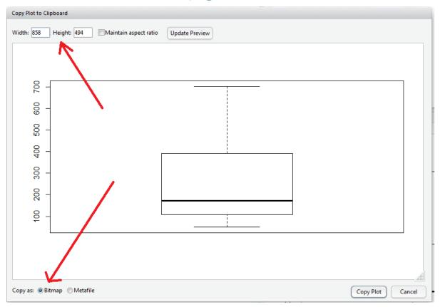
Options for the creation of the image include the dimensions of the image and the precise format \ encoding, in this case the defaults are adequate as a bitmap is a suitably versatile format. Click the Copy Plot button to copy the image to the clipboard. The image can now be pasted into any application that can make use of a bitmap, such as Powerpoint, Word, Excel of Paint:
