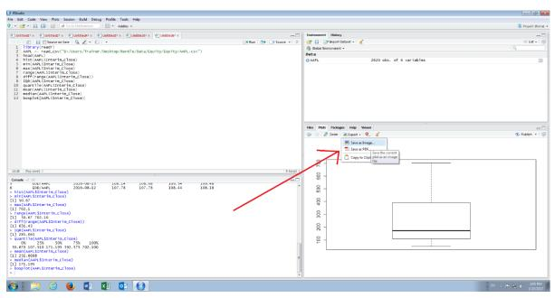
In the drop-down there are several options to export an image from a plot, although the most versatile is to copy the visualisation to clipboard as an image for pasting into a plethora of third party applications, such as Word, via the established Copy \ Paste mechanism familiar to Windows users.
